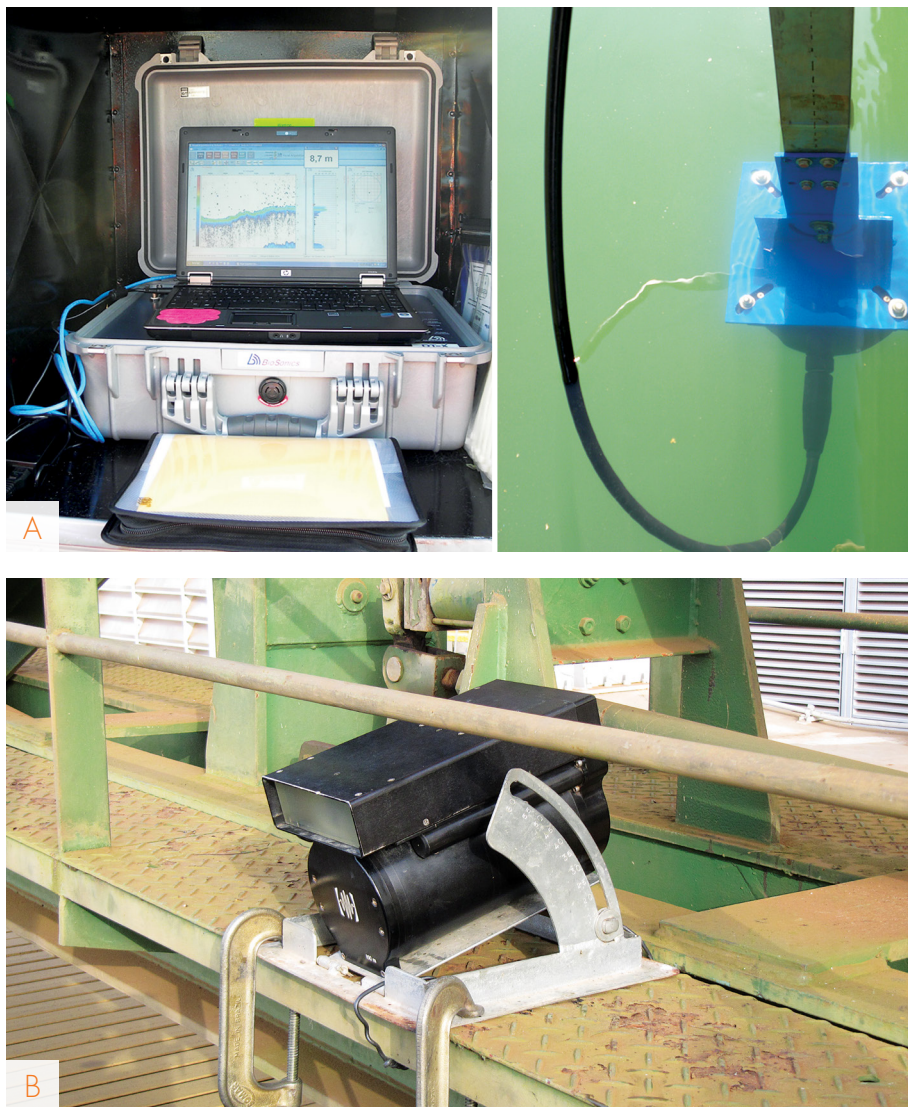
FIGURE 8 – Digital scientific echosounder (Biosonics Inc.) used to evaluate the distribution of fish in the tailrace of Três Marias Dam (A). On the left, surface unit connected to a computer; on the right, transducer attached to the side of the vessel, 50 cm above water surface, and connected to the surface unit. Dual-frequency IDentification SONar (DIDSON; Sound Metrics) used to evaluate fish density in São Simão and Amador Aguiar II dams (B). Photo B: Alejandro Giraldo
