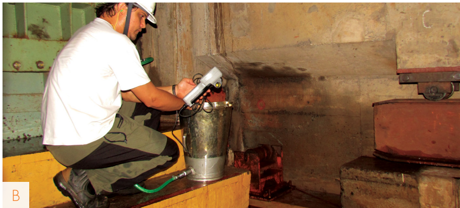
FIGURE 8 – Metal bucket, with a bottom valve that connects a hose to another valve in the draft tube hatch (A), for measuring dissolved oxygen and water temperature (B).
